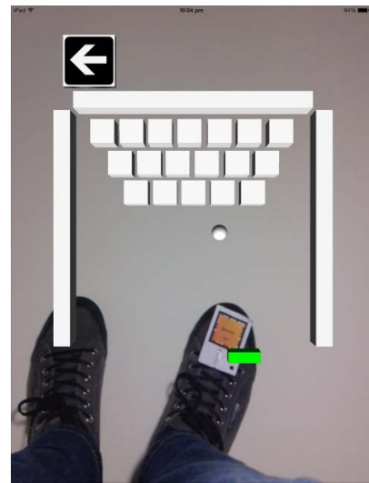
Fig. 5. AR-kanoid running on the iPad. The paddle turns green indicating that the AR marker on the foot is being tracked.
