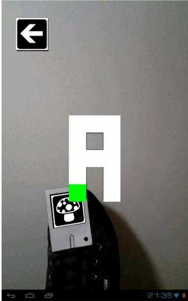
Fig. 4. The Alphabets running on an Android Tablet. The virtual ‘mushroom’ indicates that the system is tracking the movements of the player’s foot.
