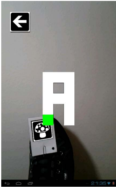
Fig. 4. The Alphabets running on an Android Tablet. The virtual ‘mushroom’ indicates that the system is tracking the movements of the player’s foot.
